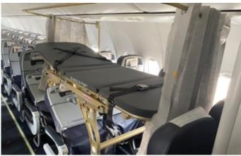
Airliners can be used for medical services with permanent or flexible installations.
