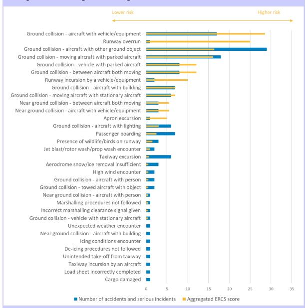
The number of occurrences for which an event was identified and the cumulated safety risk of these occurrences are provided for each type of aerodrome and ground handling operational safety event. A yellow bar in the graph, which is considerably longer compared to the underlying blue bar, indicates a low number of occurrences contributing to a high risk.
