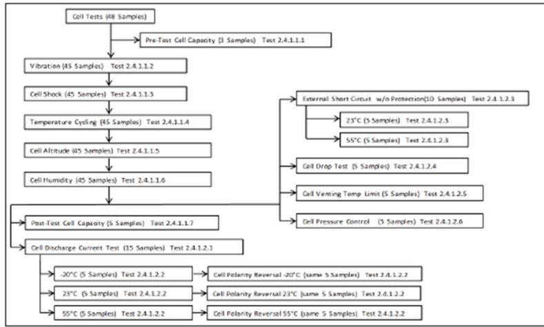
**Figure 2-25: Cell Test Sequence**
