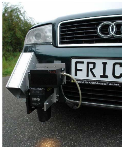
LUX Laser Scanner Attached to ika Audi
