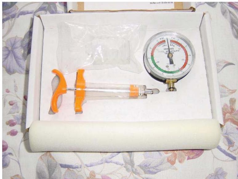
*Figure 53: Hodges tester for gasoline volatility assessment.*
