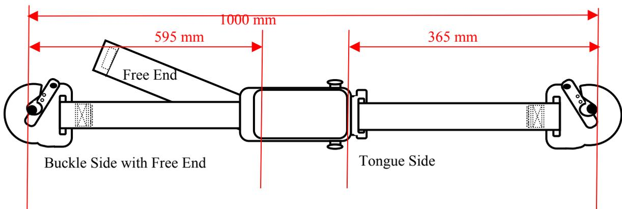
Figure B.1.5. Schematic of the belt dimensions in the Static Test Fixture
