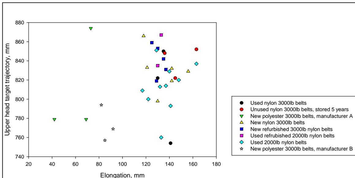
**Figure 16. Graph showing head trajectory with elongation of belt**
