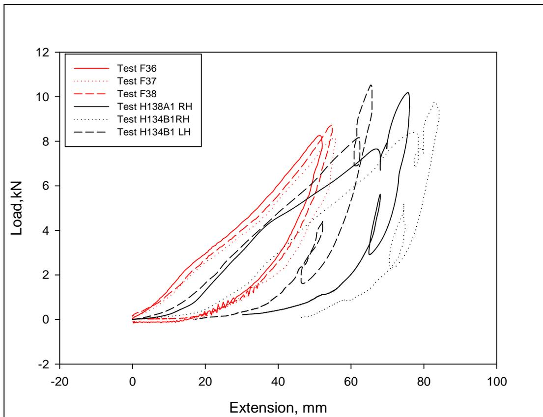
**Figure 22. Comparison of force profile from dynamic testing (black) and the feasibility test rig (red) for the tongue part of belts for new nylon belts from manufacturer A**
