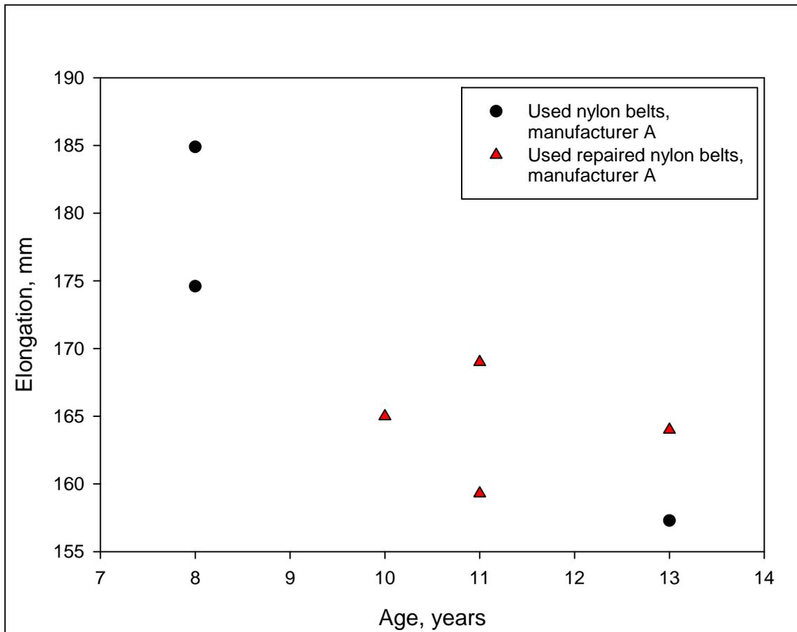
**Figure 10. Graph of elongation versus age for 2000lb belts at 26.6 kN static load**
