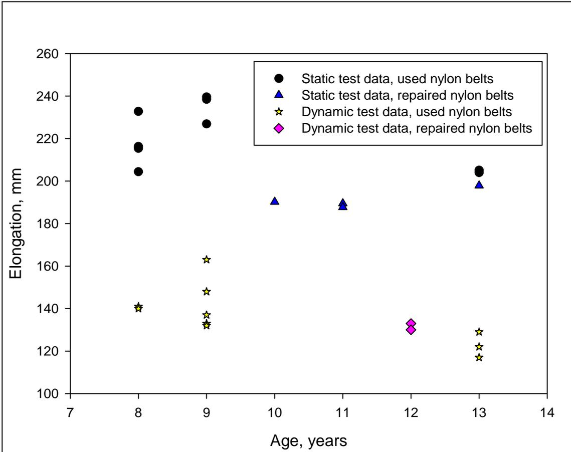
**Figure 13. Comparison of static and dynamic test results for 2000lb belts**
