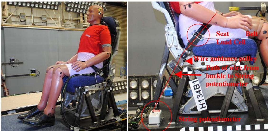
Figure B.4.3. Photograph of dummy installation into the rigidised seat and instrumentation location
