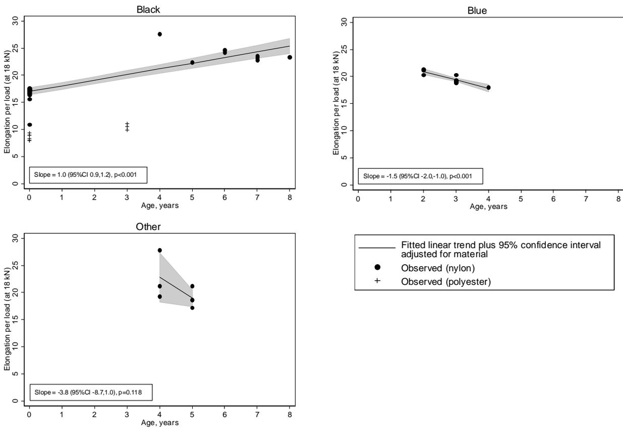
**Figure 38 Fitted linear age trend for elongation per load at 18 kN and strength 3000, by belt colour**
