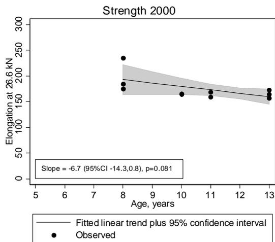
Figure 40 Fitted linear age trend for elongation at 26.6 kN and strength 2000
