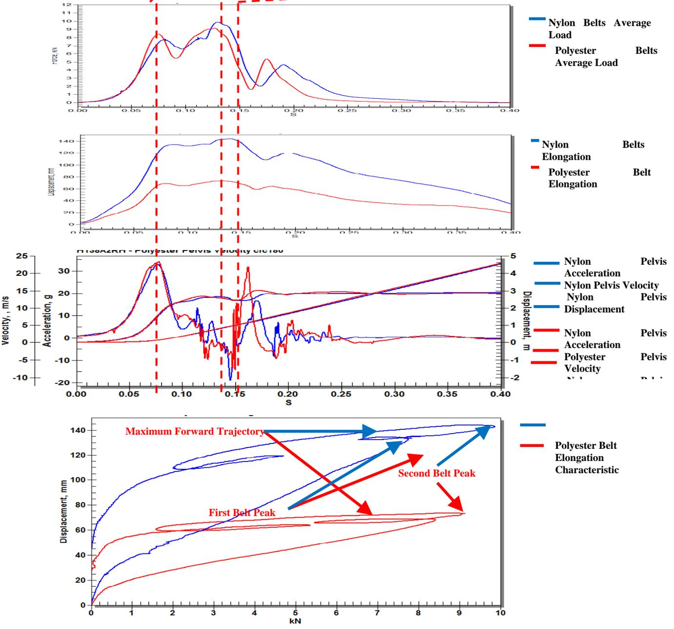
Figure B.4.9. Belt Loads with Dummy Kinematics and Loading Mechanisms
