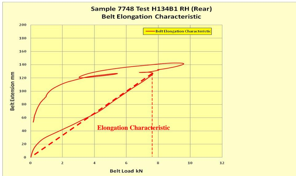
**Figure 6. Definition of Seat Belt Elongation Characteristic used in Statistical Analysis**
