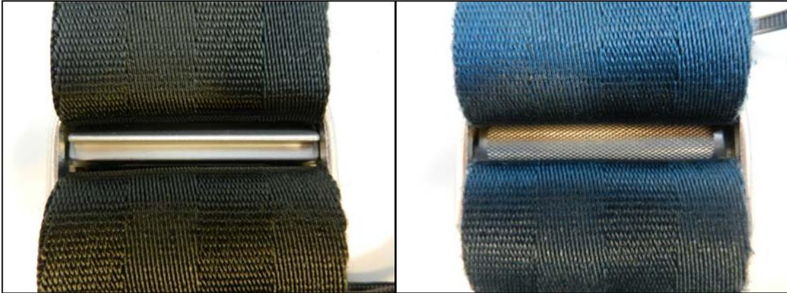
**Figure 14 a) Stepped profile buckle slide bar (left) and b) knurled cylindrical slide bar (right)**
