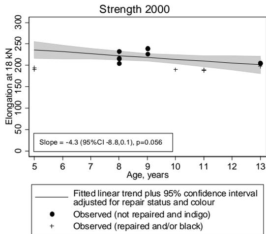
Figure 39 Fitted linear age trend for elongation at 18 kN and strength 2000
