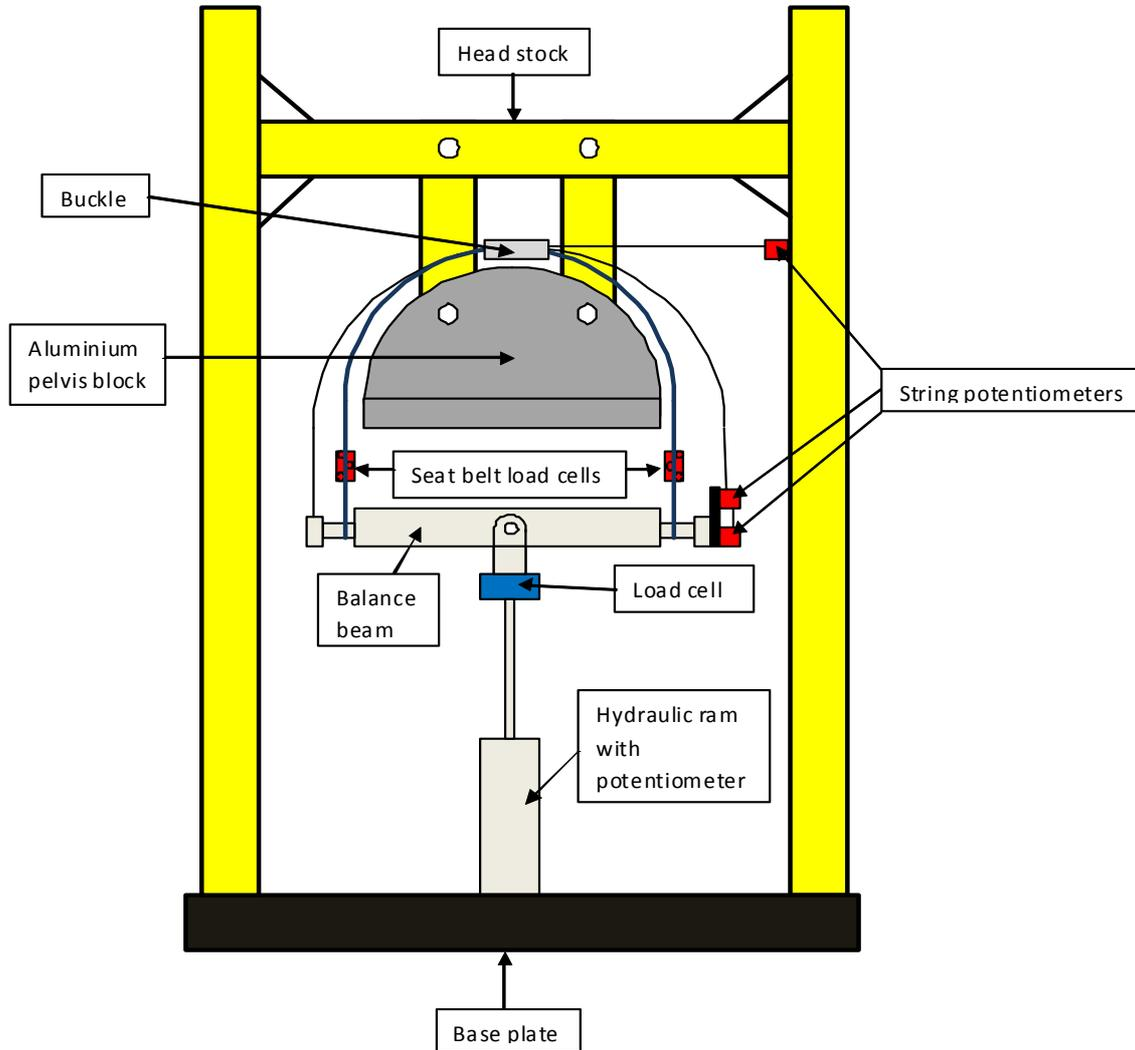
**Figure B1.2. Schematic of static test rig**
