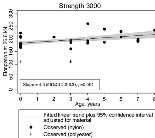
**Figure 34** Fitted linear age trend for elongation at 26.6 kN and strength 3000
