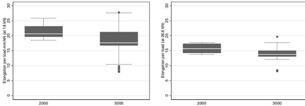
**Figure 32** Box and whisker plot of elongation per load at 18 kN (left) and 26.6 kN (right) by strength
