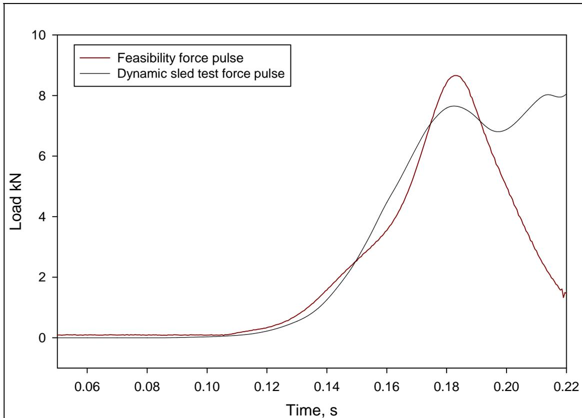
**Figure 21. Comparison of force pulse from dynamic sled test with that achieved in the feasibility rig**
