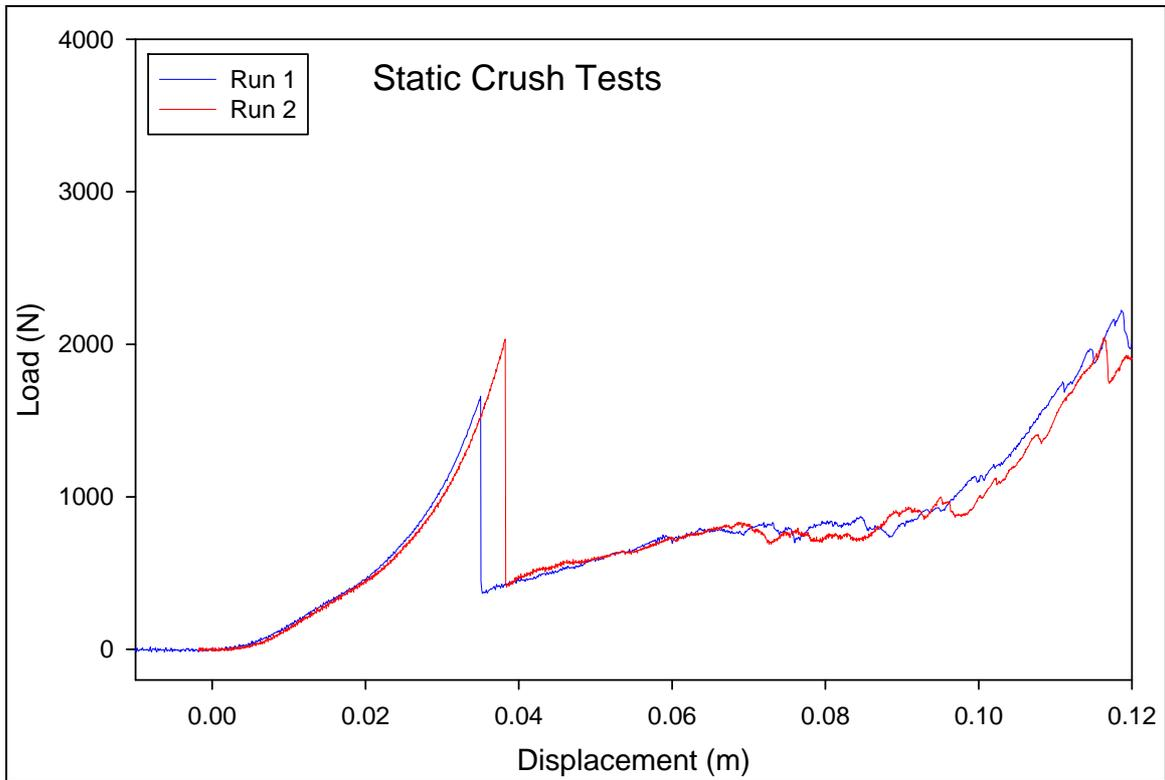
**Figure C.1. Static load-displacement profile for the energy absorber assembly used in the feasibility test rig Phase 1 and Phase 2 (115 mm crush can)**
