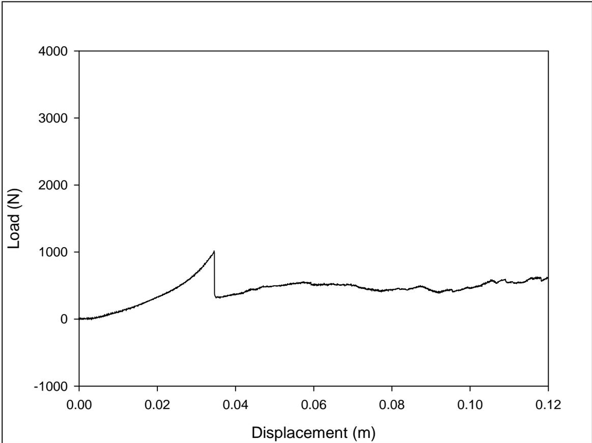
**Figure C.2. Static load-displacement profile for the energy absorber assembly used in the feasibility test rig Phase 2 (150 mm crush can)**
