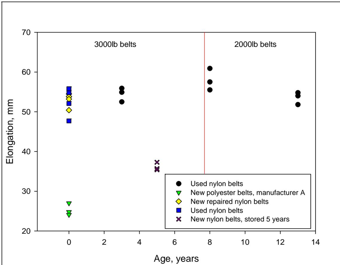
**Figure 23. Graph of elongation versus age for the tongue side of 2000lb and 3000lb belts tested in the feasibility rig**
