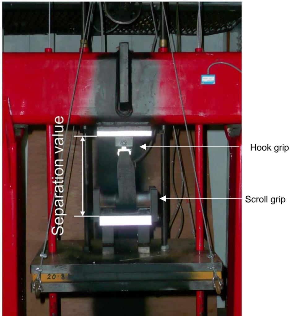
**Figure 25. Testing arrangement for Phase 2 tests**
