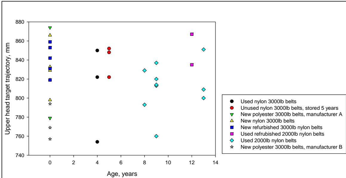
**Figure 15. Graph showing head trajectory with age of belt**
