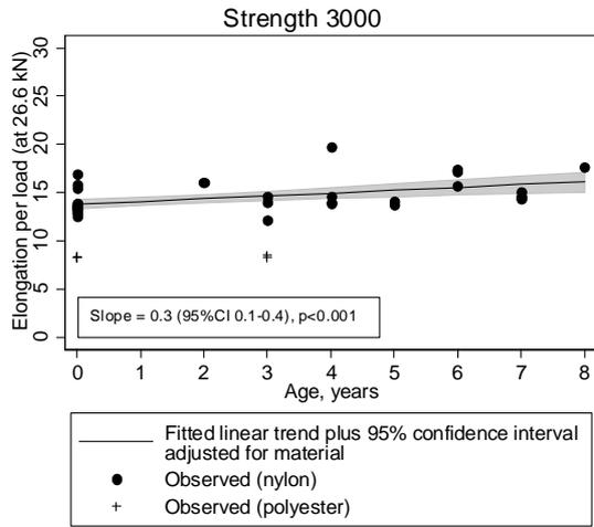
**Figure 37 Fitted linear age trend for elongation per load at 26.6 kN and strength 3000**
