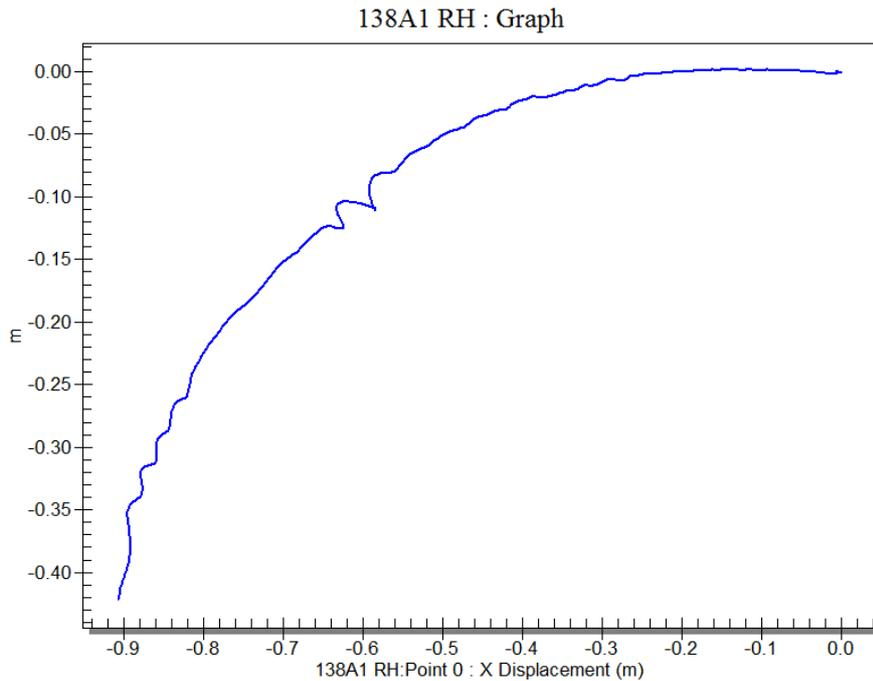
**Figure B.4.7. Graph of upper head trajectory of dummy**
