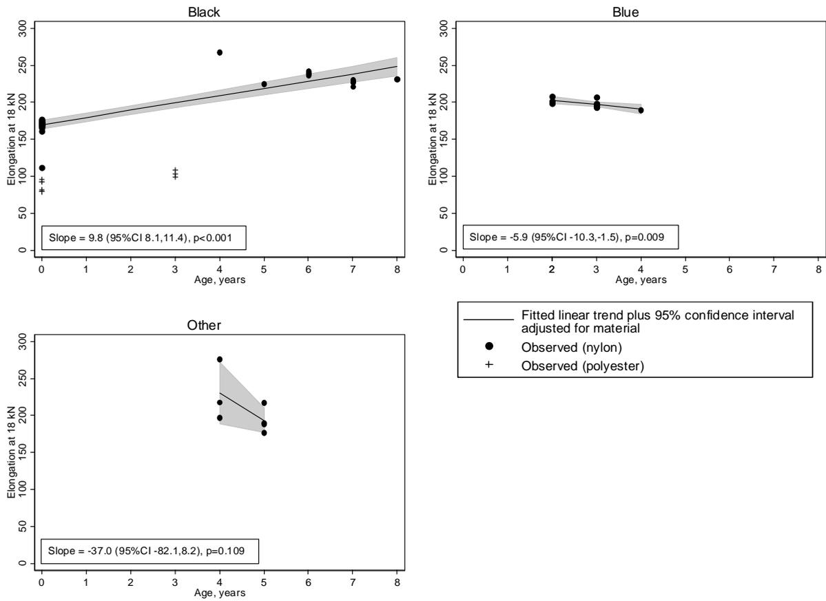
**Figure 35 Fitted linear age trend for elongation at 18 kN and strength 3000, by belt colour**
