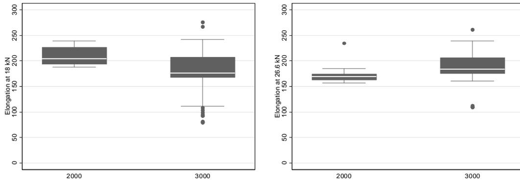
**Figure 31** Box and whisker plot of elongation at 18 kN (left) and 26.6 kN (right) by strength
