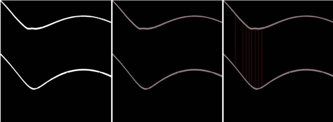
**Figure 19. Analysis conducted by HSL in-house software.** From left to right: *thresholding to remove background noise, insertion of red reference lines, measurement of reference line separation*
