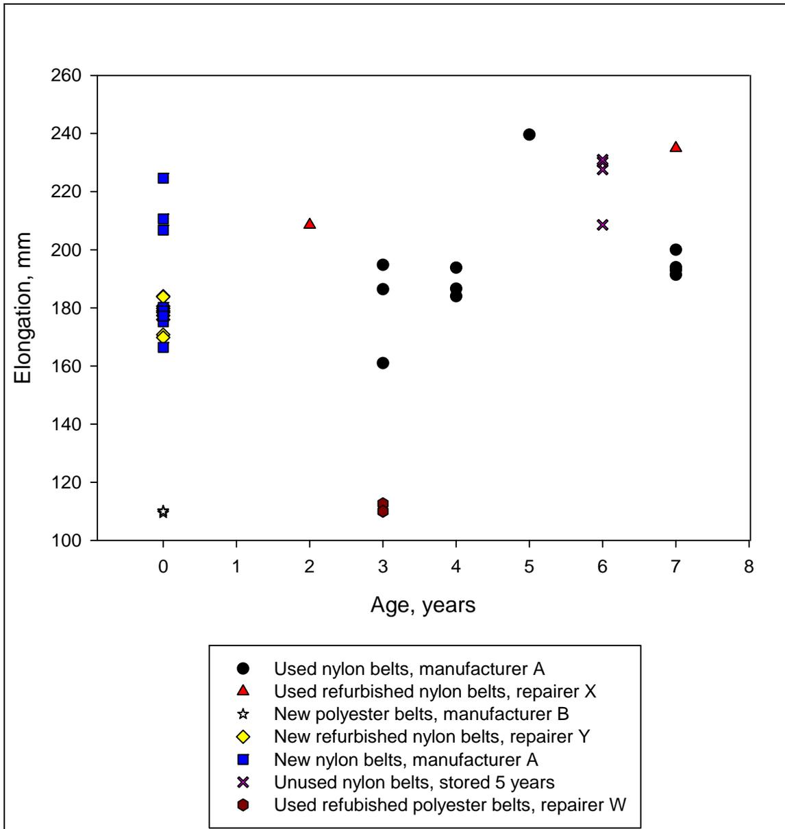
**Figure 9. Graph of elongation versus age for 3000lb belts at 26.6 kN static load**
