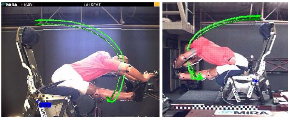
Figure B.4.6. Head disappearing behind flailing arms for the RH and LH seating locations
