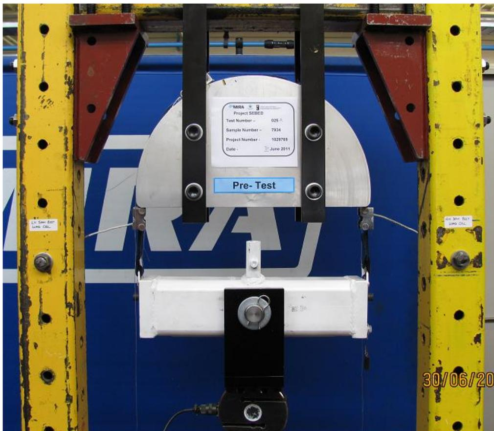
**Figure 3. Photograph of the Test Set-up showing Pelvis Block, Seat Belt Attachments and Balance Beam**
