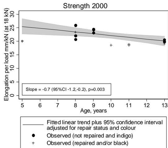
**Figure 41 Fitted linear age trend for elongation per load at 18 kN and strength 2000**
