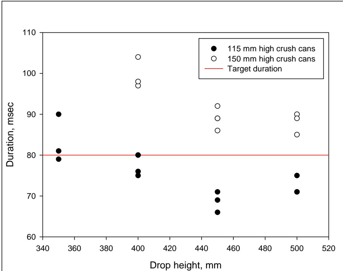
**Figure 27. Graph showing the relationship between drop height and duration for fixed 300mm sample length**
