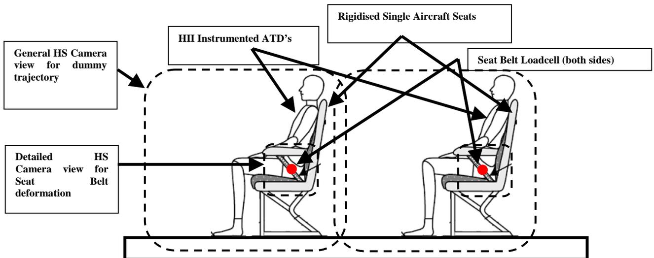
Figure 4. Schematic of reverse acceleration sled
