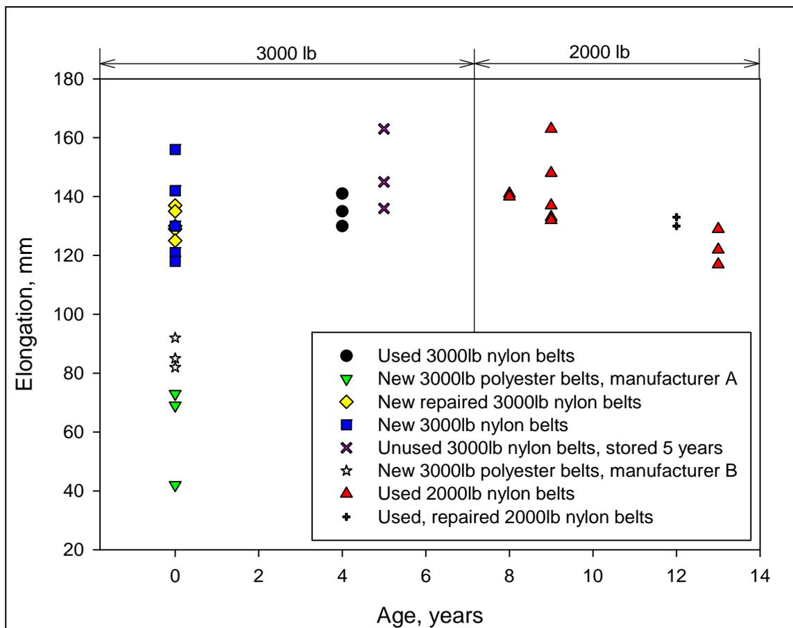
Figure 11. Graph of elongation versus age for belts tested dynamically
