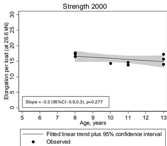
**Figure 42 Fitted linear age trend for elongation per load at 26.6 kN and strength 2000**
