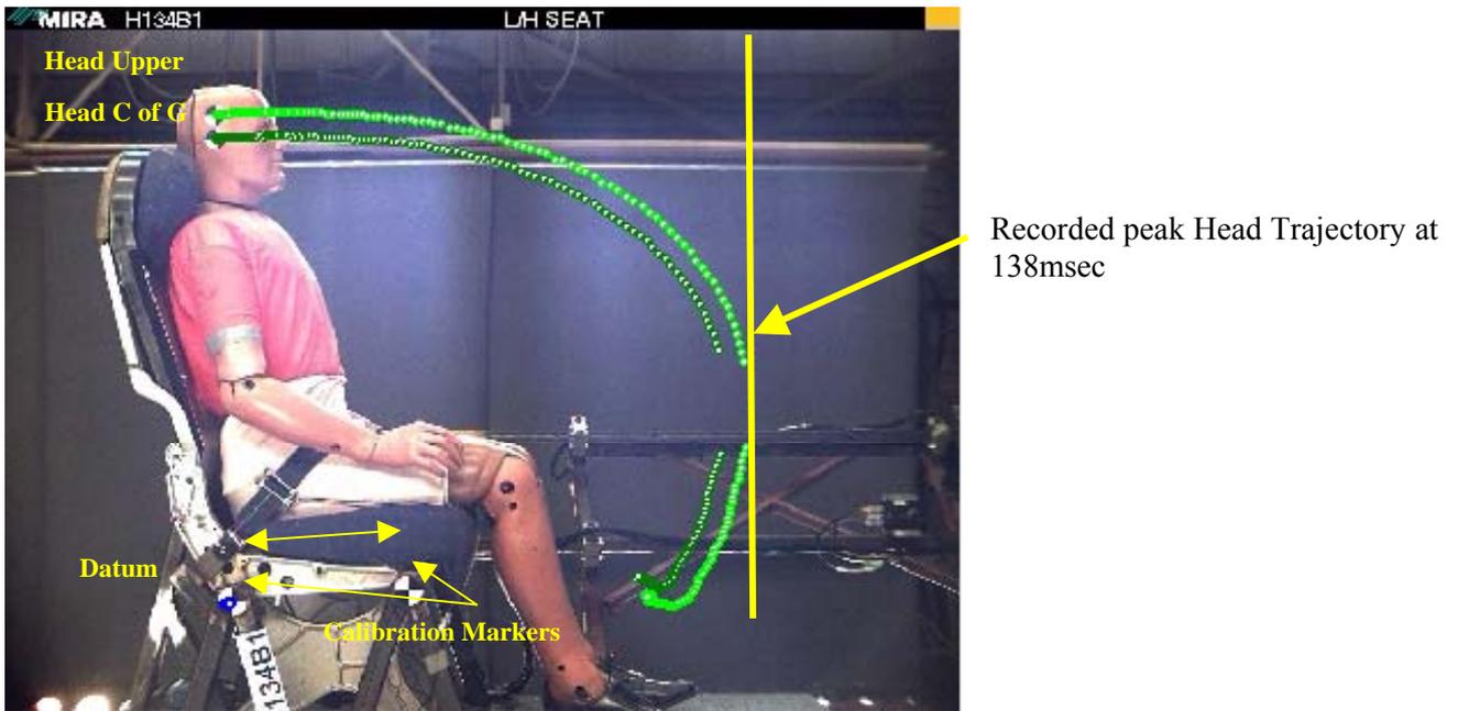
Figure B.4.5. Head Trajectory analysis showing Peak Trajectory location immediately prior head marker disappearing behind flailing arms
