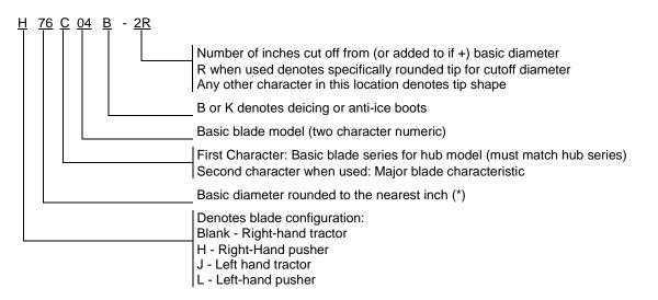
(\*): Diameter limits are nominal diameters of the assembled propeller. They do not include the + or - 1/8 inch manufacturing tolerance the FAA allows for propellers with a basic diameter of less than 14 feet (426,72 cm).
