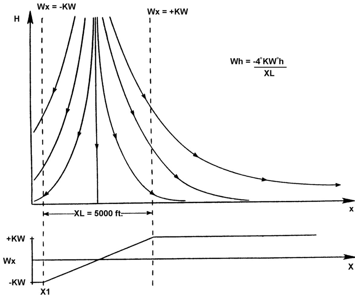
**Figure 1 — Wind Model Used in Guidance Studies**
