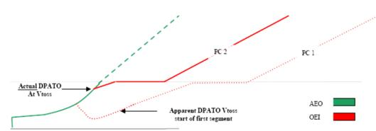
Figure 8: Using Cat A data; actual and apparent position of DPATO ( $V_{toss}$  and start of first segment)
