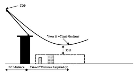
The main difference is that drop down below the level of the take-off surface is permitted. In the drop down phase, the Category A procedure ensures deckedge clearance but, once clear of the deck-edge, the 35 ft clearance from obstacles relies upon the calculation of drop down. Item (b) of AMC1 CAT.POL.H.205(b)(4) is applied.
