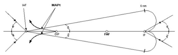
Figure 3: Holding pattern & race track procedure
