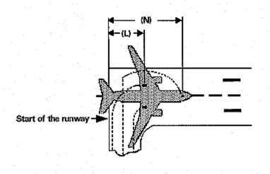
Where the aeroplane manufacturer does not provide the appropriate data, the calculation method given in (b) should be used to determine the alignment distance.
