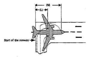
Where the aeroplane manufacturer does not provide the appropriate data, the calculation method given in (b) may be used to determine the alignment distance.
