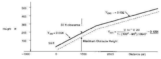
(2) Assumed engine failure height 200 ft
